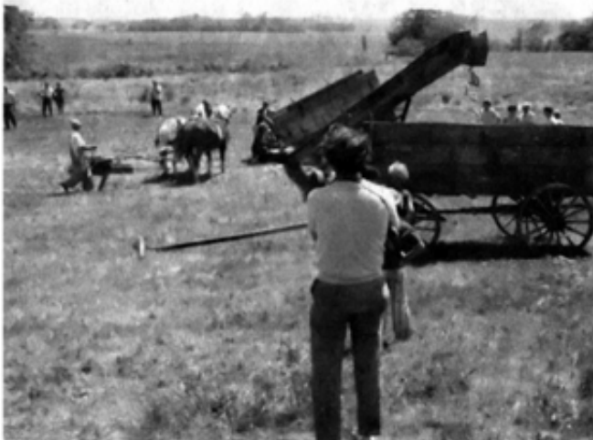
Horses were also used to elevate corn into wagons, just as it used to be done, through the use of horse power, which, as shown here, used a team of horses walking in a circle pulling an arm which in turn moved the gears for power.
